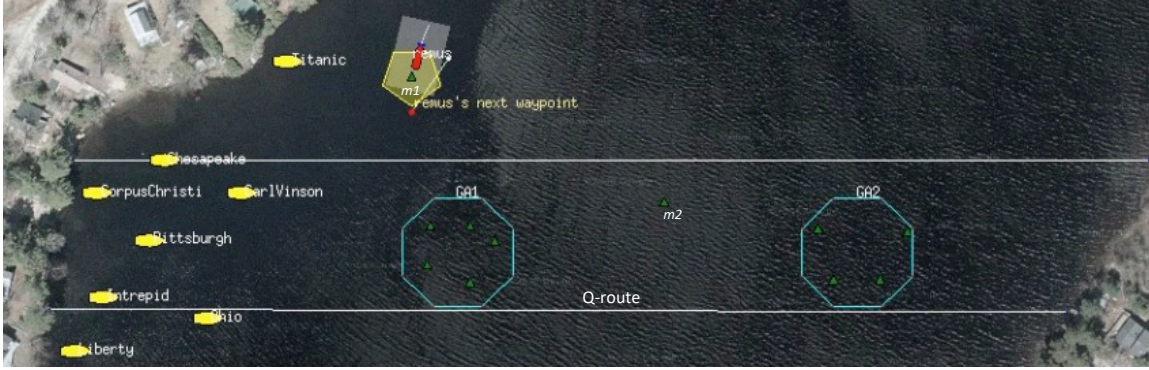
Figure 3. Simulation of the mine clearance domain in Moos IvP. The Q-route extends from the left to the right side of the map. Shipping (shown in yellow) awaits on the left side of the map, and the Remus platform (in red) encounters a mine ( m1 in the pentagon) as it transits to the GA1 location.
