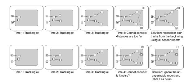
*Figure 2.* Anomalies due to order dependency (top) and noise (bottom) in the simulated object tracking domain. Reports for objects in the middle gray area do not specify the object's color (here represented by 'x' and 'o'), thus any object within a short range could possibly account for the detection.
