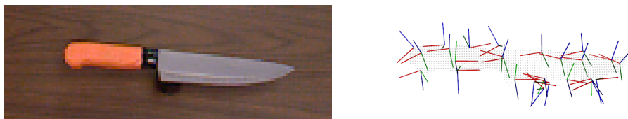
Figure 2. Left: knife; Right: Grasp candidates across the knife. Cognitive affordances can serve as a normative constraint when selecting one of the many grasp possibilities.
